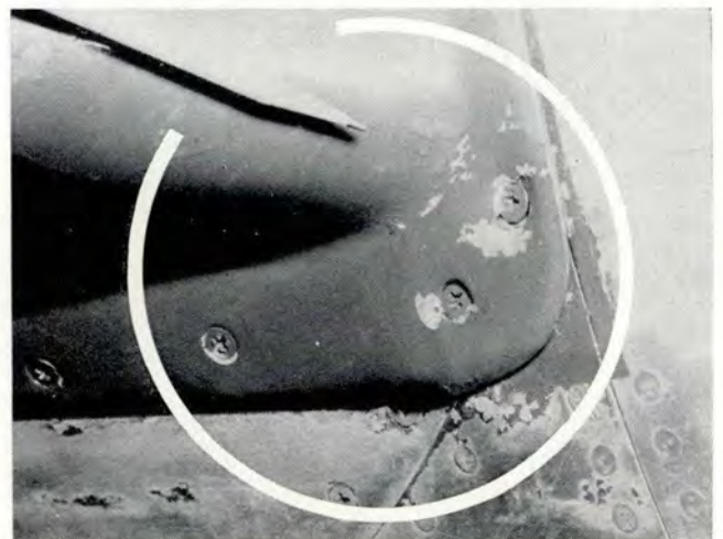
Above, circle shows underside fuselage skin surfaces buckled on left side. False leading edge is pulled away from screws at root. Below, right false leading edge is pulled away from screws at root.
