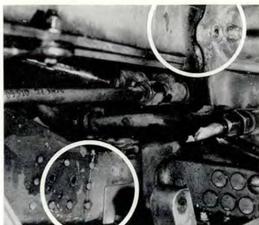
Lower left shows left main gear wheel well revealing breaks and pulled rivets. (Plumbing removed for examination.) Above, close-up of left main gear wheel well showing breaks and failed bolt of wing fitting to forward spar. (Plumbing removed.) Below right, wing fitting to forward spar attaching bolts sheared and separated.
