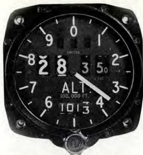
Pilot's view of Smith's Altimeter showing window and pointer system.
