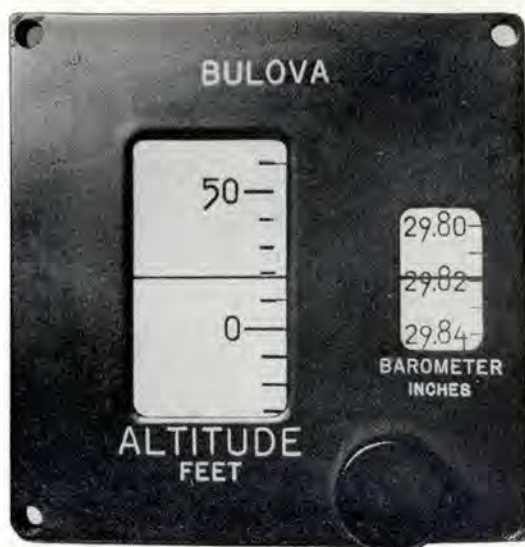
Pilot's view of Bulova altimeter showing tape method of presentation.
